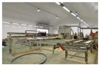
TIMBER CUTTING, CROSS-CUTTING AND TONGUE AND GROOVE PROFILING WORK
